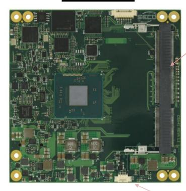
Ext. FAN Connector SO-DIMM Slots
